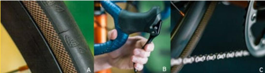
**A** is for Air: Having properly inflated tires helps prevent flats. Check the sidewall of your tire for the recommended tire pressure. While you're checking the air, take the opportunity to ensure your quick-release levers and thru axles (if you have them) are properly tightened as well. Then, before you ride, make sure you have your patch kit and pump with you.
